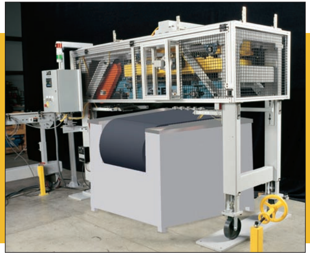
Guard in place
