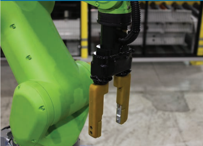
End of Arm Tool with Urethane-Over-molded Fingers
