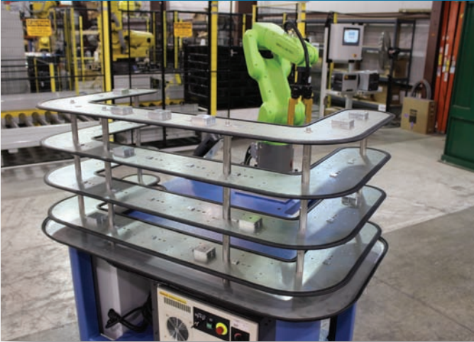
C-Shaped Work Piece Queue with Drip Pan
